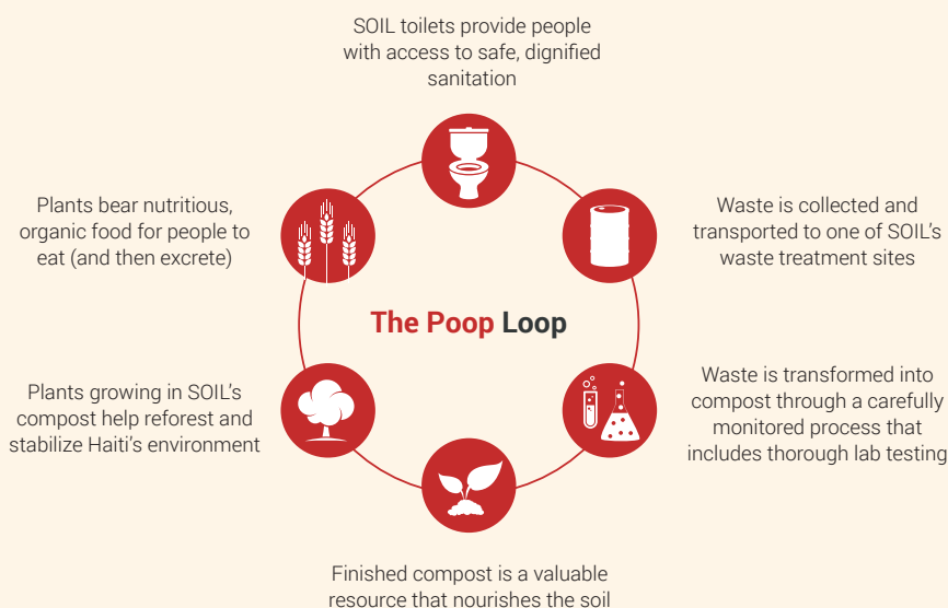
Figure | Ecological Sanitation Method
