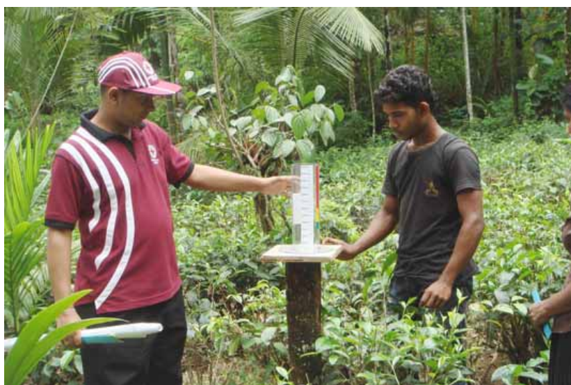
Sri Lanka Red Cross Society staff explaining the usage of the rain gauge to a community member in Rathnapura, Sri Lanka.
