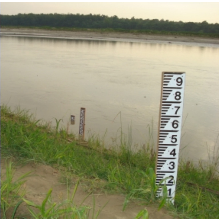
Water- level gauge
